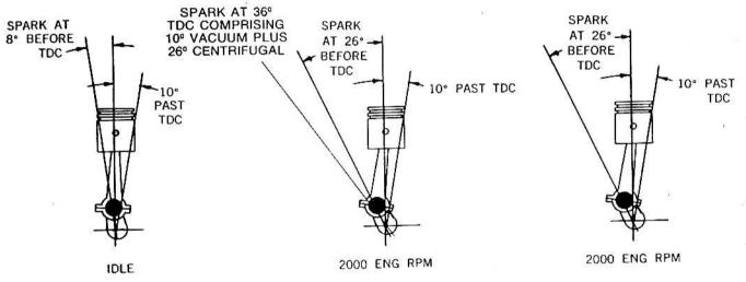
Engine speed is relatively slow allowing sufficient time for flame spread and complete burning.
